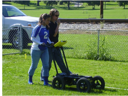
Students using ground-penetrating radar.
